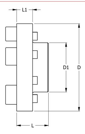
D = 520 D1 = 250 L = 210 L1 = 68 Max bore = 150 Torque (N m) = 21200
